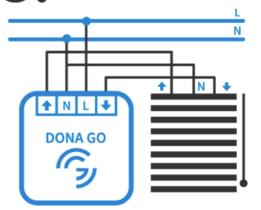
Connect the device in accordance with the diagram
